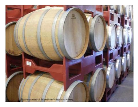
Plastic barrel racks are also corrosion resistant, recyclable, and gentler on barrels and cellar floors.
